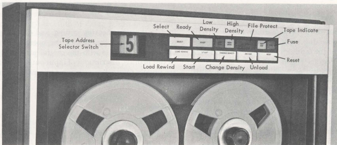
Figure 72. Operating Keys and Lights, IBM 729 II Magnetic Tape Unit
