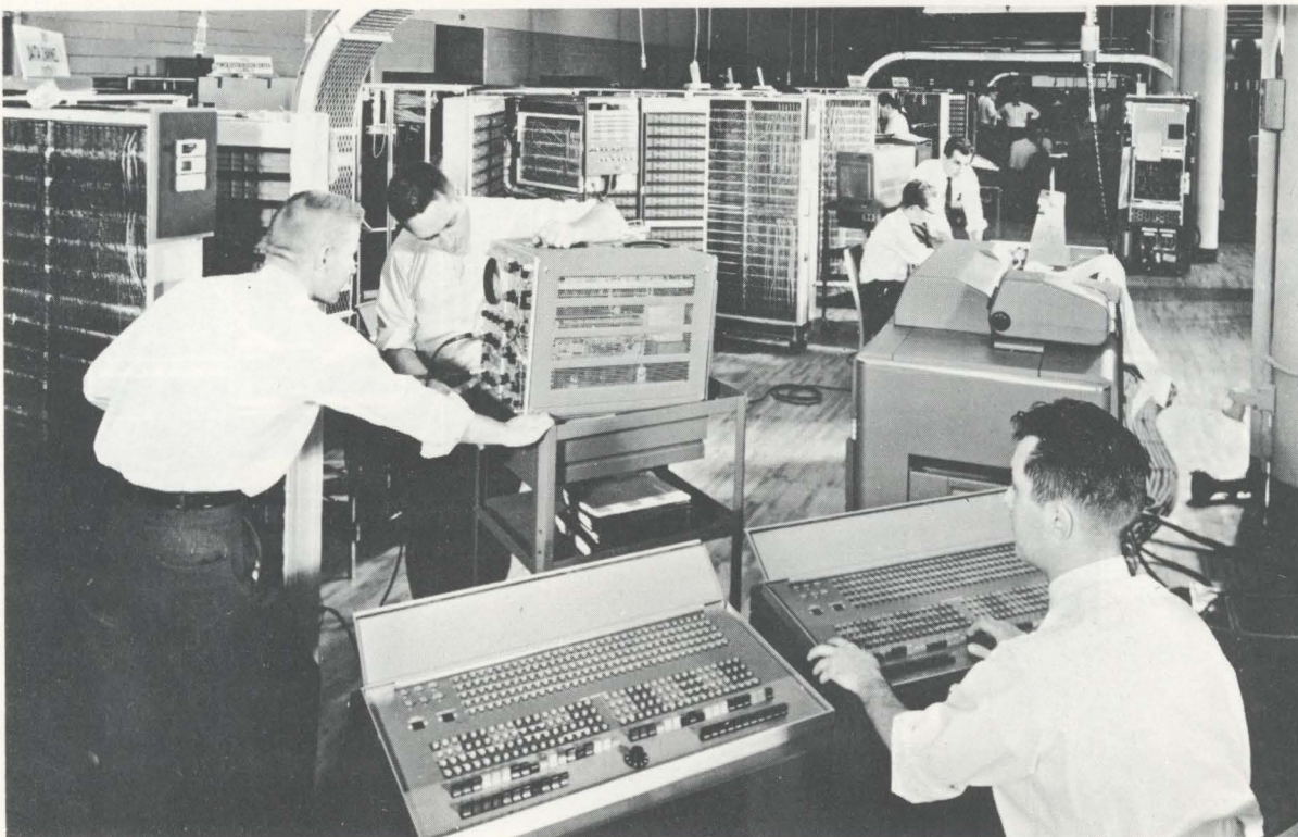
Figure 2. In-manufacture Test of Large-scale IBM Data Processing System
